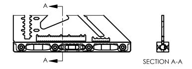
STEP 2: REMOVE THE HEEL TO EXPOSE THE BLADE OF THE SQUARE AND LEVEL VIAL.
