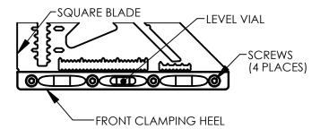
STEP 3: HEEL REMOVED SHOWING LEVEL VIAL IN POSITION.
