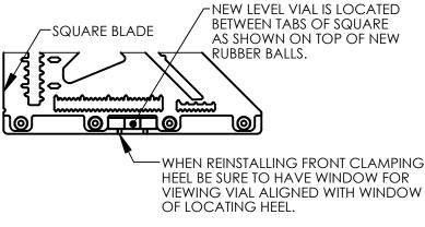
STEP 6: SQUARE ASSEMBLED WITH SECTION VIEW SHOWING VIAL CORRECTLY INSTALLED.
