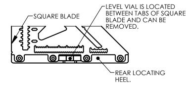
STEP 5: HEEL REMOVED SHOWING LEVEL VIAL IN POSITION.
