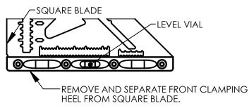
STEP 4: RUBBER BALLS ARE LOCATED BEHIND LEVEL VIAL AND CARE NEEDS TO BE TAKEN TO BE NEW RUBBER BALLS ARE POSITIONED IN DRILLED POCKETS AS SHOWN
