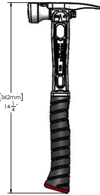
M1 FRAMING HEAD INSTALLED ON M4 FINISH HANDLE WITH CURVED GRIP TOTAL WEIGHT: 1 LB 14 1/3 OZ (862 GRAMS) M1M-M4-C & M1S-M4-C
